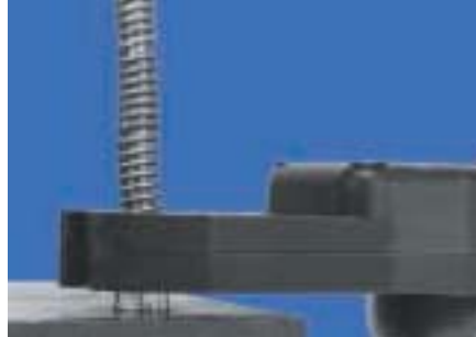
Slide the tool onto the fastener and press the lever to run the fastener down.
