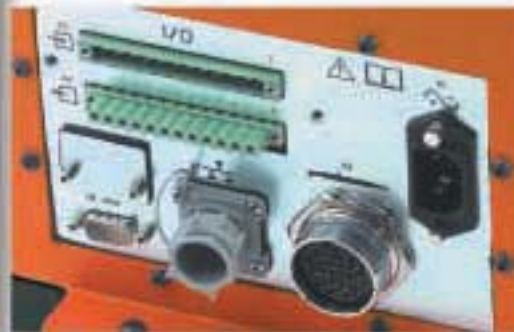
24 volt inputs and output connectors on the I/O version controller are compatible with existing TME accessories.
