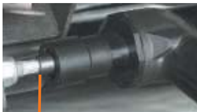
Hold socket fits over bolt and prevents it from rotating.
