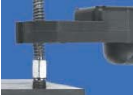
The 47ET tube nut wrench alternates the direction of rotation each time the lever is actuated. When rotating in reverse, the socket will stop at the open position.
