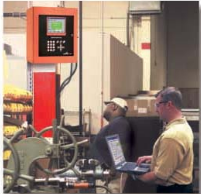
TMEs that are out of reach can be re-programmed or analyzed through an Ethernet crossover cable with TM-COM, TM-COM1, or TM-COM1M.
