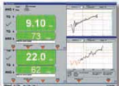
You can also launch multiple sessions to the same TME or TMEM I/O so you can monitor the Run Screen and the Oscilloscope at the same time.
