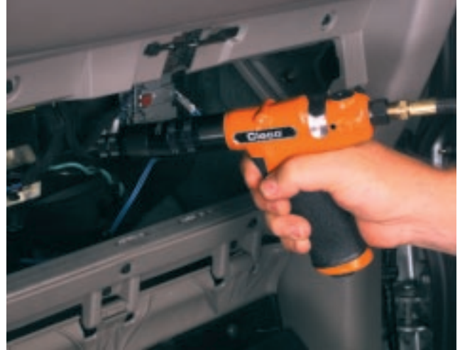
Hidden, but easy to access, torque adjustment reduces on line tampering.
