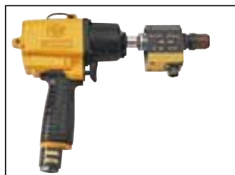
Reading the torque applied by pneumatic oil pulse wrenches.
